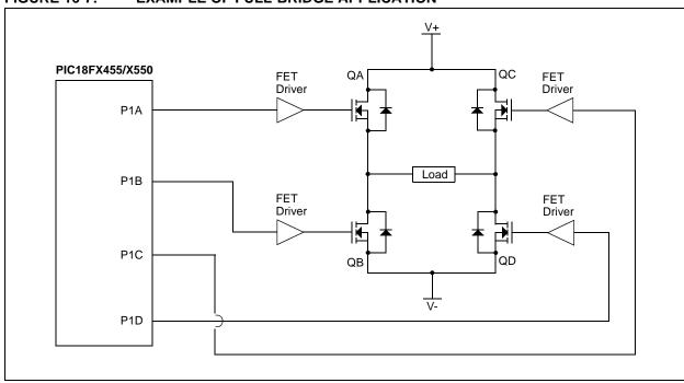
FIGURE 16-7: EXAMPLE OF FULL-BRIDGE APPLICATION
