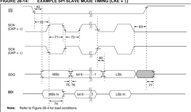
FIGURE 28-14: **EXAMPLE SPI SLAVE MODE TIMING (CKE = 1)**
