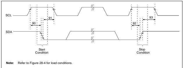
TABLE 28-21: MASTER SSP I<sup>2</sup>C™ BUS START/STOP BITS REQUIREMENTS
