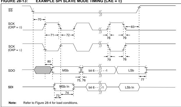
FIGURE 28-13: **EXAMPLE SPI SLAVE MODE TIMING (CKE = 0)**
