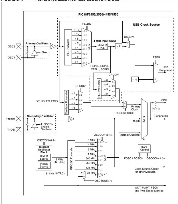
FIGURE 2-1: PIC18F2455/2550/4455/4550 CLOCK DIAGRAM
