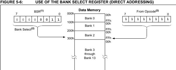
Note 1: The Access RAM bit of the instruction can be used to force an override of the selected bank (BSR<3:0>) to the registers of the Access Bank.
