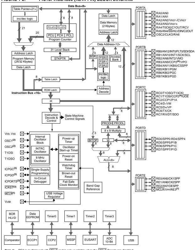
FIGURE 1-2: PIC18F4455/4550 (40/44-PIN) BLOCK DIAGRAM
