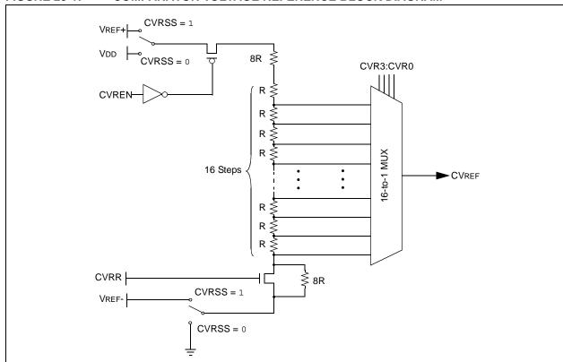
FIGURE 23-1: COMPARATOR VOLTAGE REFERENCE BLOCK DIAGRAM
