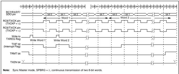
FIGURE 20-12: SYNCHRONOUS TRANSMISSION (THROUGH TXEN)
