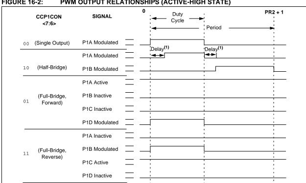
**FIGURE 16-2:** PWM OUTPUT RELATIONSHIPS (ACTIVE-HIGH STATE)
